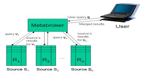
Fig. 2 Meta-broker Architecture
